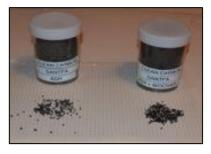
Above – (L) 100% ash and (R) 80% ash + 20% Biochar. The poultry litter ash was granulated into a flowable and low dust product suitable for application with cropping equipment.
